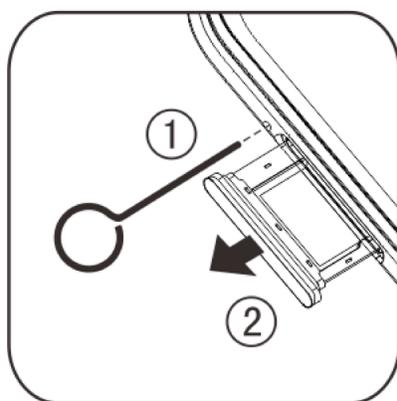
2. Make the metal face of the Nano card (SIM1/SIM2) or Micro SD card face downward, with the oblique angle corresponding to that of card tray. Put the Nano card (SIM1/SIM2) or Micro SD card into the card slot according to the direction indicated by arrows of the diagram.
