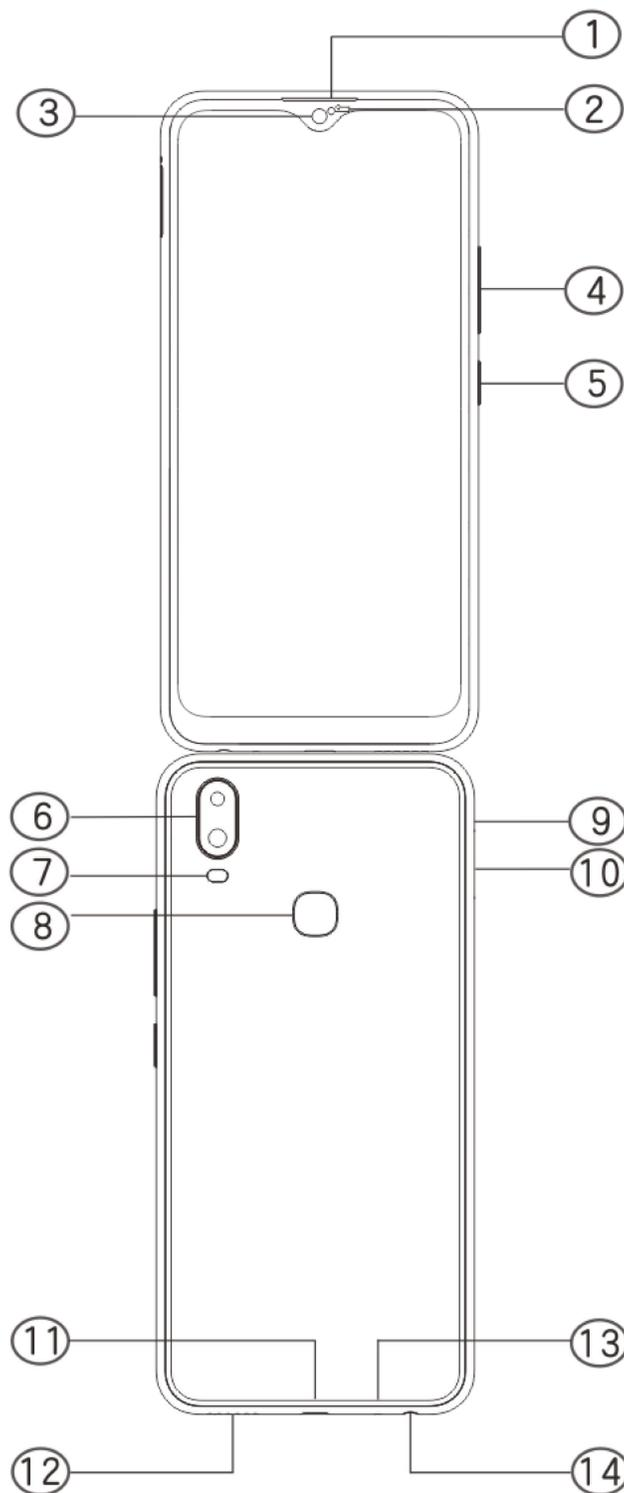
1. Receiver; 2. Light & Proximity sensors; 3. Front camera; 4. Volume button; 5. Power button; 6. Rear camera; 7. Rear flash; 8. Fingerprint sensor; 9. Pin port; 10. Card tray; 11. USB port; 12. Speaker; 13. Microphone; 14. Headset port.
