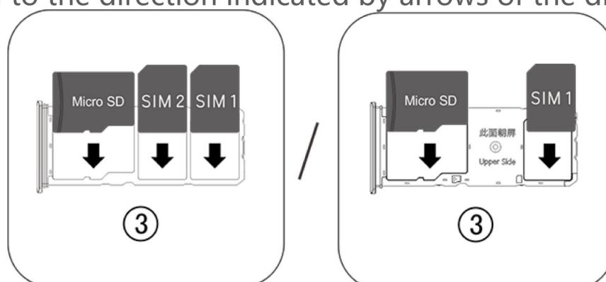
3. Touch screen facing up, follow the direction of the arrow to install the tray (with Nano card or Micro SD) into the phone.
