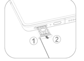
2. Place your nano-SIM card into the SIM 1 or SIM 2 holder in the direction of the arrow as shown in the illustration. Make sure to align the angled corner to the notch on the holder.
