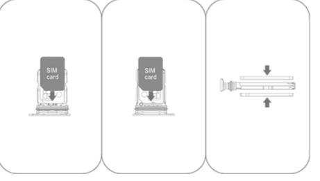
3. Hold your device face up, and then slide the tray all the way into the slot in the direction as indicated by the arrow.
