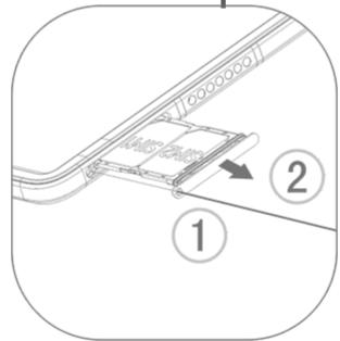
2. Place your nano-SIM card into the SIM 1 or SIM 2 holder in the direction of the arrow as shown in the illustration. Make sure to align the angled corner to the notch on the holder.
